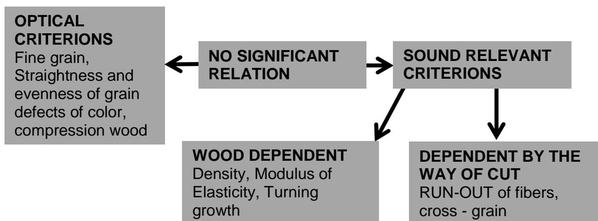
To get more insight in the physical properties of tonewood, the suppliers should provide their products with the same measured values which, in order to be comparable, should be independent of the sample's dimension.
